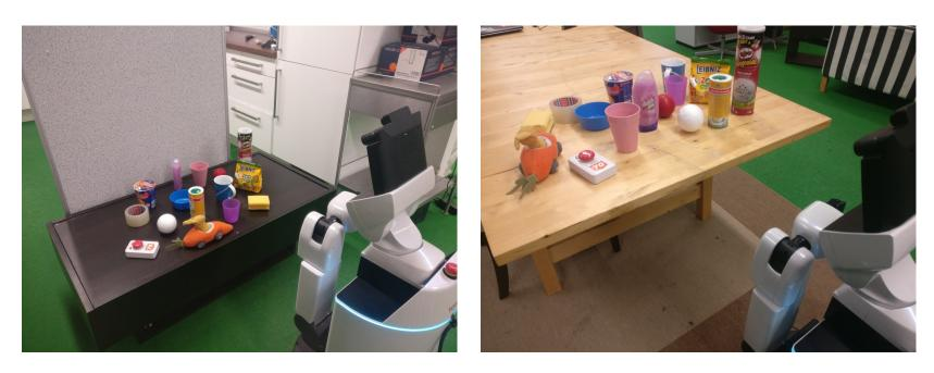
For evaluation, we recorded a grasping primitive for the HSR and performed experiments involving grasping 15 different objects from two surfaces - an ordinary dining table and a living room table.
