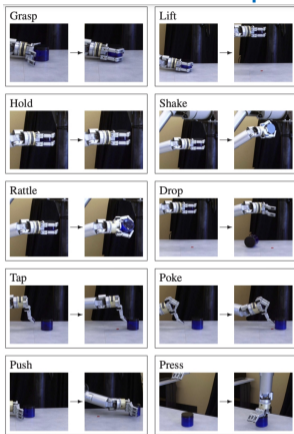
Fig. 2: Before and after images of the 10 exploratory behaviors that the robot used to learn about the objects.
