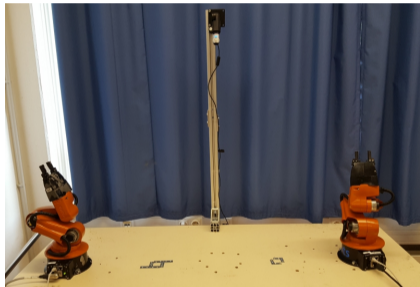
A setup for estimating positions of placed objects with a camera in one of our labs. Here, the error model is estimated by manually measuring object positions.
